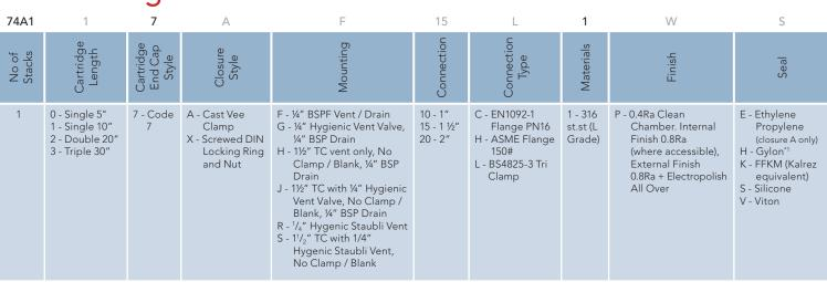
Example: 74A117AF15L1PS = **74A Series**, 1 x 10" Code 7 cartridge, cast vee clamp, ¼" BSPF vent/drain, BS4825-3 Tri Clamp connections, St. Steel construction with 0.4Ra clean chamber and electropolished externally, silicone seal.
